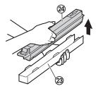
16 Insert each toner cartridge (S) in the appropriate color slot.
